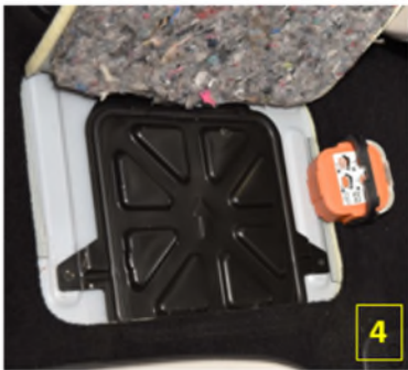
First: Uncover the Service Disconnect access cover.
