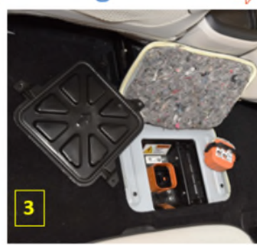
Third: Remove the Service Disconnect.
