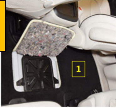
First: Uncover the Service Disconnect access cover.
