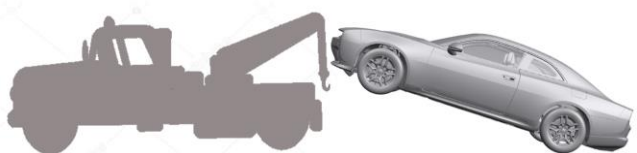
DO NOT TOW WITH WHEELS ON THE GROUND
