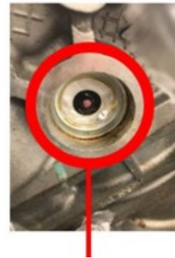
Overheated Red Sensor +255°F Coolant Temp
