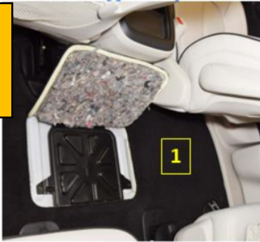
1 First: Uncover the Service Disconnect access cover.
