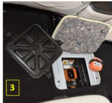
3 Third: Remove the Service Disconnect.
