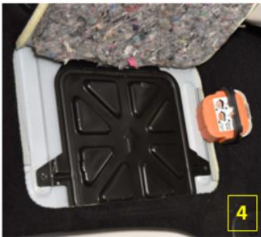
1 First: Uncover the Service Disconnect access cover.
