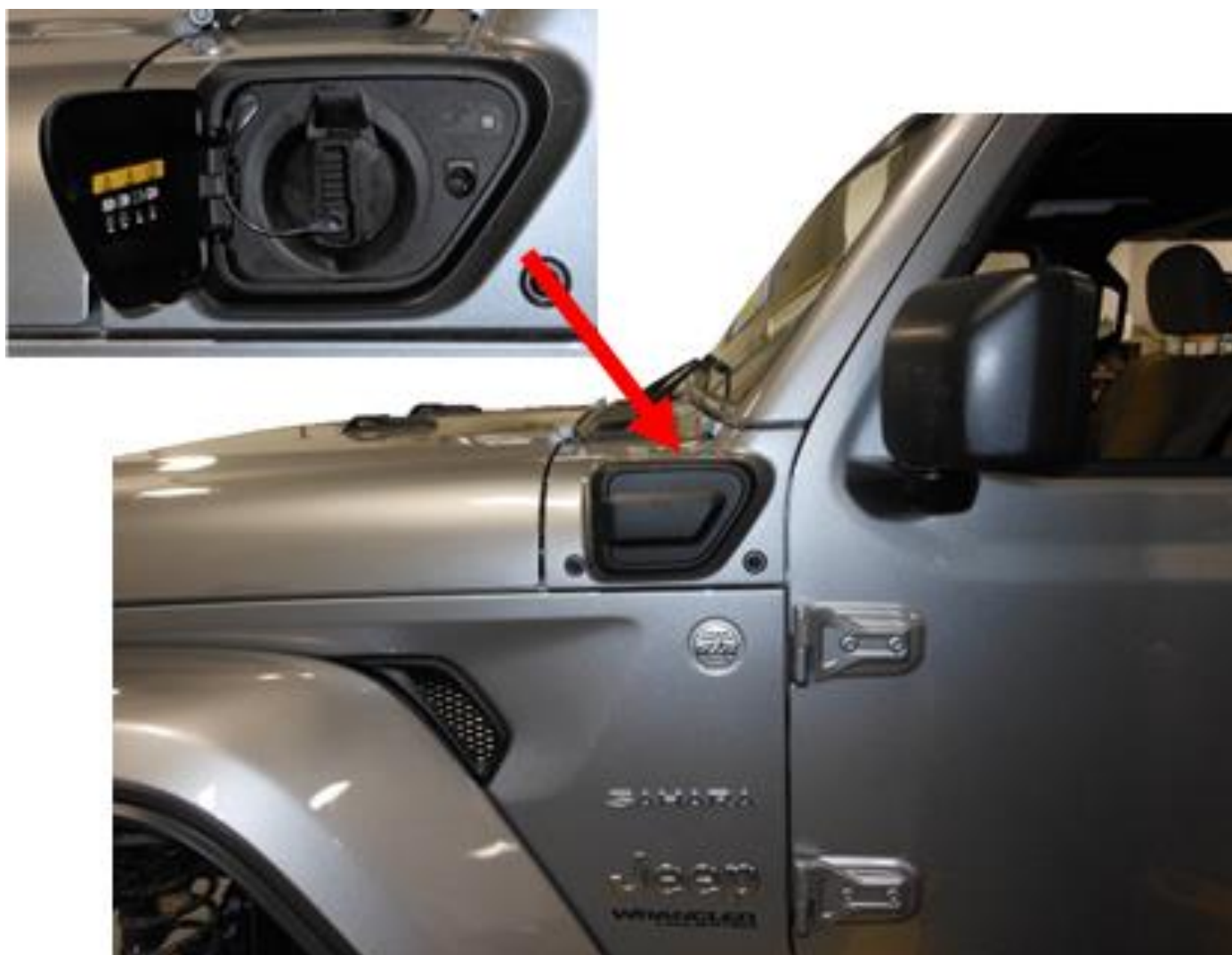
A charge port, which is located at the driver-side cowl side panel.
