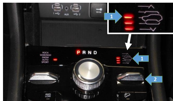
1- Normal Ride Height 2- Ride Height Toggle Switch
